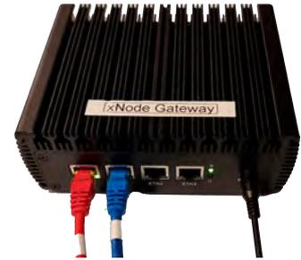
b) Next, plug one end of the short blue ethernet cable to the ETH1 port. Plug in the other end to the LAN port of the "PoE Brick" which acts as the power supply to the Lucius radio unit.
