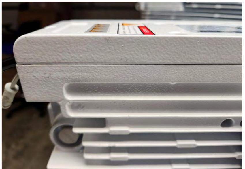
**Note- The cover must fully close to seal properly against weather!**
