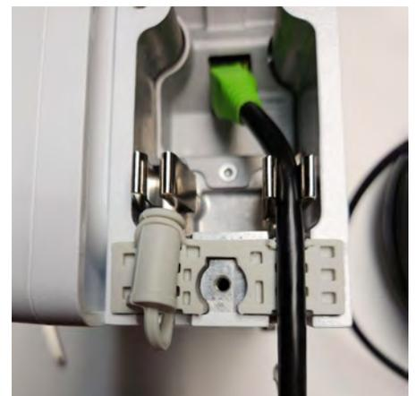
3. Pass the ethernet cable through the weather plug retaining clip
