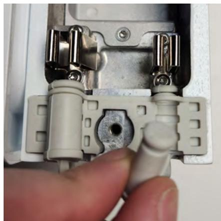
2. Remove the smaller diameter weather plug on the right side
