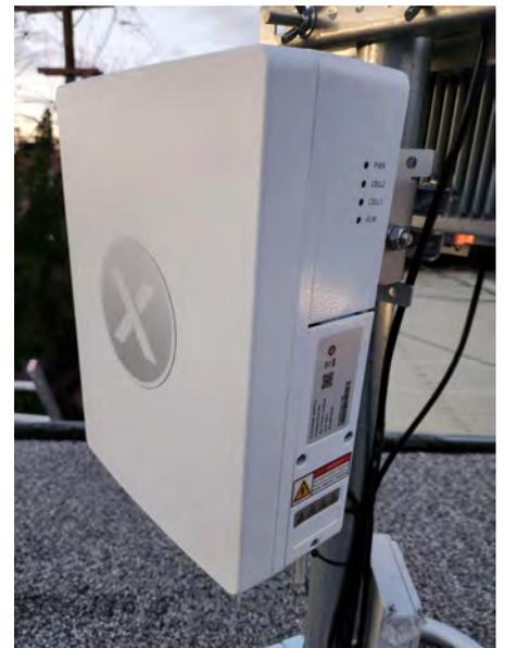
d) Connect the end of the 150' ethernet cable (black cable) into the interior ethernet port on the Lucius radio:
