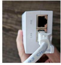
**Step 3:** Connect the longer ethernet cable to the PoE Wi-Fi ethernet port as shown below:
