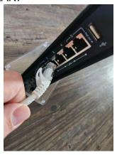
**Step 2:** Connect the PoE adapter port labeled PoE using the longer ethernet cable:
